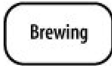
Figure 14-4. A rectangle with rounded corners and the name in the center is the most common way to draw a state 状态名
